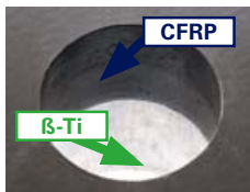
Hole Produced by Circular Interpolation
